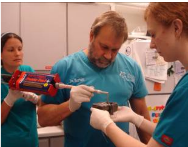
Figure 2: Applying epoxy on satellite transmitter
